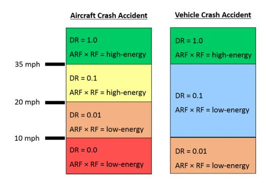
**Figure 3.** *DOE Standard 5506-2007 interpretation of aircraft and vehicle crash assumptions.*
